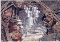
Next was the removal of the stock **Q**uadrajet carburetor in favor of a Holley throttle plate. A standard carburetor adapter was used to adapt the Holley throttle plate to the Q-jet intake manifold. Then, the Technocarb mixer was bolted to the Holley throttle plate. A fuel block-off plate was mounted in place of the stock mechanical fuel pump.
