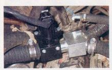
7 This is the digital power-control stepping motor, which controls flow of propane between the converter and the mixer. Think of this as a precision gate valve that controls the vapor.
