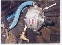
Next, a step critical to the driveability of the vehicle: The fuel regulator/converter (arrow) must be mounted as shown above for the diaphragm inside to function properly. We made a support bracket from scrap metal we had lying around the garage. The fuel lock-off solenoid is visible below the converter. Notice the blue heater hose we used to tie the converter into the vehicle's cooling system. The heat from the coolant is necessary for the liquid propane to change into a gas.
