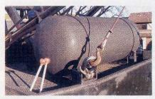
The next step was mounting a DOTapproved tank. Rockstar Trux in San Jose mounted our 60-gallon tank under the wrecking boom on the back of the flatbed. We decided on this mammoth vessel for two reasons. First off, it was cheap-we found it for sale in a local newspaper, and second, it provided a large enough reserve of propane for a whole weekend of 'wheeling. Forklift tanks are a good option for those with limited space in which to mount a tank.
